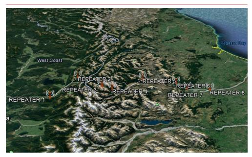
"The noticeable difference in using this simulcast repeater is the seamless roaming. We could actually see radios roaming between repeaters to the strongest signal mid conversation. This is a step change from old technology where you had to finish a conversation before the radio would move to a nearer repeater."
