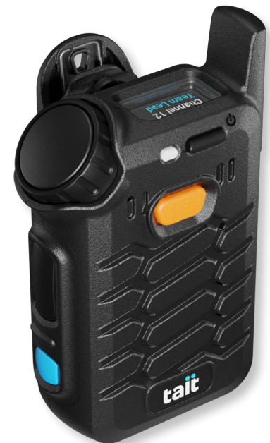
Rotary dials and buttons provide tactile and audible feedback for heads-up operation.
