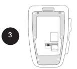
Make sure the inside of the device is clear of any dust and dirt, specially the grey area shown, to ensure the water-tightness of the device.
