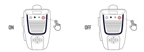
Turn on by pressing the Power button until the green LED turns off. Turn off by first pressing the Power button until "Shutdown?" appears on the screen, and then press the right arrow button to confirm the shutdown process. You can also shutdown the device through the main menu.
