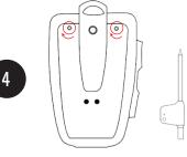
Insert the battery back into the device so that the battery contacts align and the battery label faces into the device. Then slide the battery cover back into place and screw it shut. Do not over tighten.
