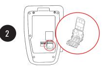
Slide the SIM card holder downward, lift the holder into an upright position and slide the SIM card into the holder. Make sure the SIM card's gold contacts face into the device and the angled corner of the card is positioned correctly (as shown in the picture on the left). Set back down the SIM card holder and slide it upwards to secure it (the SIM card should be lying flat on the device).
